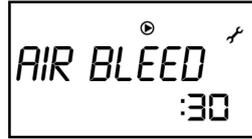
The purging cycle activates the circulator pump at an alternating rhythm to allow the displacement and purging of any air bubbles accumulated at high points of the installation using the **Pilot's** automatic purger.
