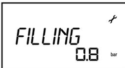
During the filling stage, the **Pilot** indicates the pressure measured in the heating circuit.
