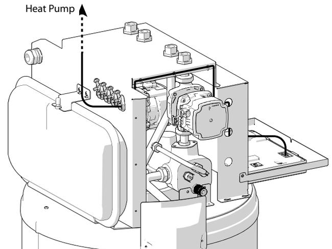
Plan for the appropriate length of cable between the pilot and the heat pump. Do not hesitate to cut the cable to the appropriate length to **AVOID LOOPS**.
