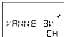
CH: the valve switches to heating (lower position)
