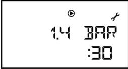
During the purging cycle, the screen indicates the countdown until the automatic stop of the cycle as well as the pressure in the circuit.
