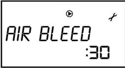
The purging cycle activates the circulator pump (and the 3-way valve if production of domestic hot water is also installed) at an alternating rhythm to allow the displacement and purging of any air bubbles accumulated at high points of the installation using the **PRIMO Pilot's** automatic purger.
