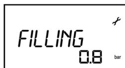
During the filling stage, the **PRIMO Pilot** indicates the pressure measured in the heating circuit.
