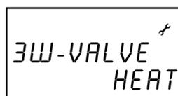
**HEAT** : the valve switches to heating (lower position)
