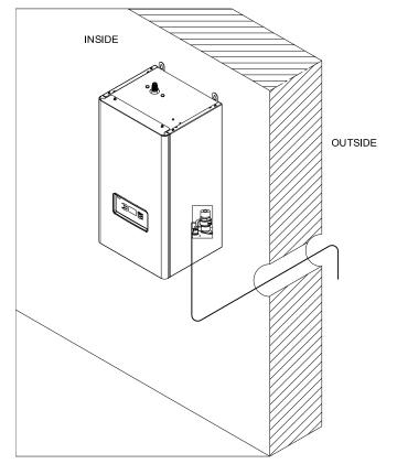
The Pilot's pressure-relief valve drainage pipe must be properly secured until the outside of the building without any pinching zone.
