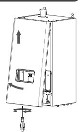
2- Pull the base of the front panel forwards, and lift the panel to unhook the pegs located at the top of the PRIMO Pilot.
