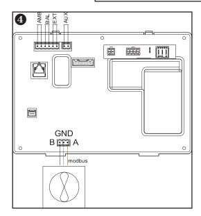
**Amb** : Ambient temperature sensor or thermostat
